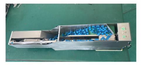
**Principle:** Through the components selection track, NG components through the reflux Belt return: The selected material is transported to the material level by direct vibration
